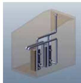
Common vertical vent/ individual sidewall air
